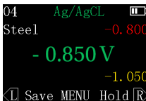
Figure 6 Corrosion Measuring Screen
